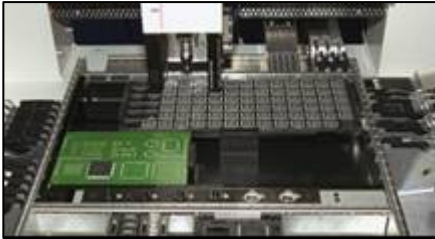
CSM771 mounted in placement area
